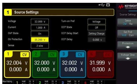
Figure 6. E36441A provides OVP, OCP, and OTP protections
